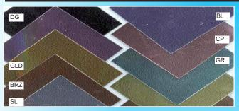
TINTED MIRRORED SHEET Reflective mirror film laminated to a 1mm black styrene sheet with a protective polyfilm. Available in a good range of colour tints. Uses range from reflective glass on architectural models to mirrors in dollhouses. Material is flexible and can be applied to curved surfaces. Cuts easily like regular styrene with the score and snap technique (score on mirrored side). Apply to surface with double-sided adhesive (STICKM), bonds to styrene or
