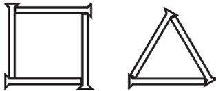
Typical methods of assembly for boxed sections
